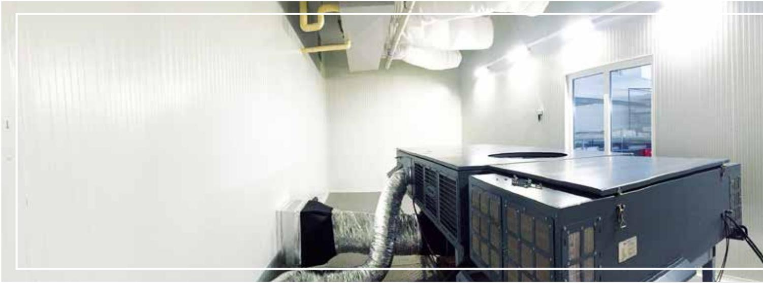
Test chambers are specially designed rooms where temperature, humidity and air speed are precisely controlled (PLC and PC).
